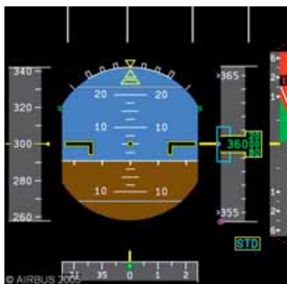
Figure 2: TCAS RA HMI without AP/FD TCAS mode
